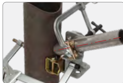
Use w/ MagSpring Clamp to join pipe at angle
