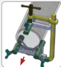
Loosen the main clamp arm.
